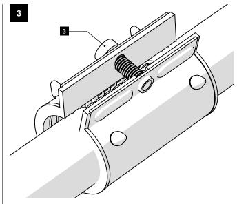
3. Tighten the screw (3÷4 Nm)
