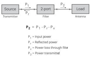
Fig. 1: Filter as element of a system.
