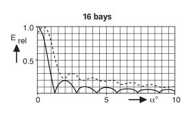
without null fill – – – – – with null fill and beam tilt
