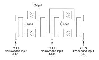
Fig. 7: Directional filter combiner with 2 modules
