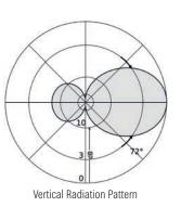
\* Radiator mounted onto a slim steel tube, tower effects not considered
