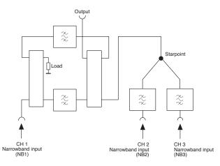
Fig. 8: Multiplexer for three channels
