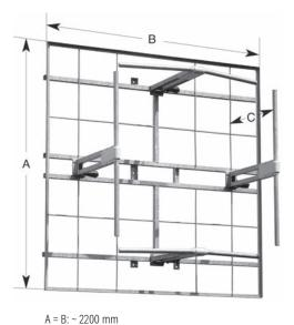
4 dipoles are arranged symmetrically in front of a reflector screen. With suitable feeding the antenna radiates circularly polarized. An isolation of 40–50 dB between horizontal and vertical pairs of dipoles is achieved through the special design. This design allows the transmission of 2 programs – horizontally and vertically polarized – independently from each other.
