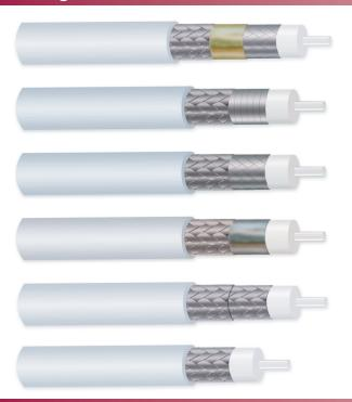
**Triple Shield** - Woven flat braid, polyemide foil, round braid. Provides >90 dB shielding effectiveness, high torque resistance, mechanically strong.
