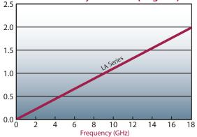
Phase stability is defined as the change in phase when the cable is bent 360 degrees around its minimum bend radius.
