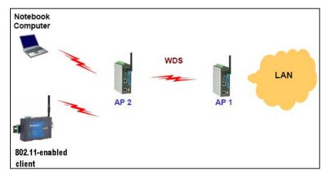
By using WDS, two or more LAN segments can be connected wirelessly. As illustrated in the above figure, a pair of wireless LAN-to-LAN bridges is used to connect two LAN segments. Since the AP is WDS-enabled, it can be used as a wireless bridge.
