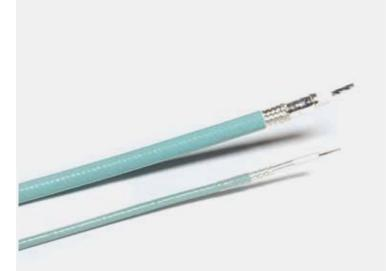
M-FLEX Microwave coaxial cables are a family of flexible cables designed to accept connectors designed for Semi-Rigid cable. Unlike other single or double braided "RG" type flexible cables, M-FLEX cables are true microwave cables capable of operating to frequencies of 26.5 GHz. The extended frequency range is the result of a precision helically wrapped silver plated copper foil inner shield. This inner shield allows for outstanding flexibility while providing 100% coverage.
