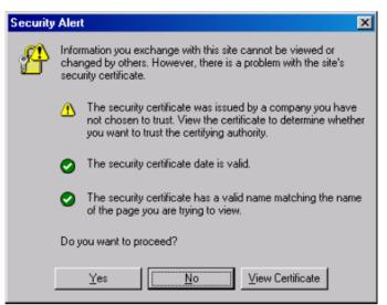
Select Yes to accept the certificate issued by Moxa IW and then enter the AWK-3131-RCC's web browser interface secured via HTTPS/SSL. (You can see the protocol in URL is https.) Then you can use the menu tree on the left side of the window to open the function pages to access each of AWK-3131-RCC's functions.
